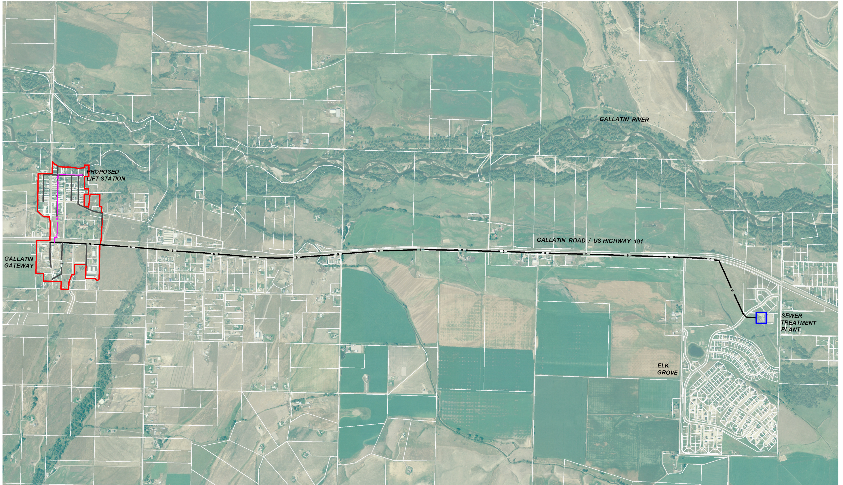
FIGURE 7.3.2B TREATMENT ALTERNATIVE T-2 GRAVITY MAIN TO UTILITY SOLUTIONS GALLATIN GATEWAY COUNTY WATER AND SEWER DISTRICT 2010 PRELIMINARY ENGINEERING REPORT (PER)
